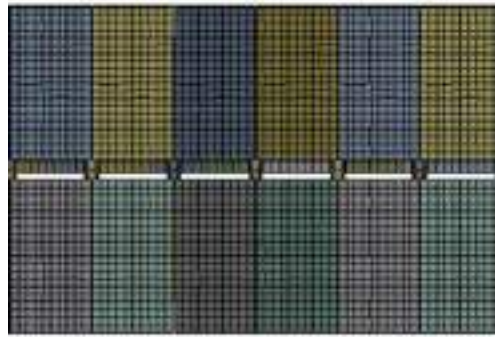
Figure 10. Shell Elements at Solar Module
