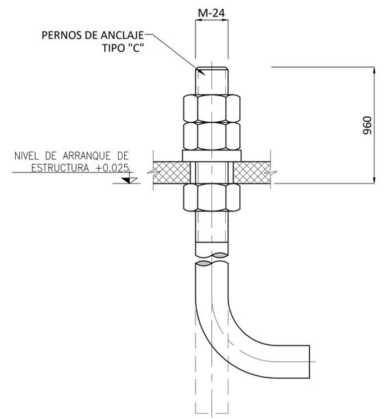
DETALLE PERNO DE ANCLAJE TIPO
