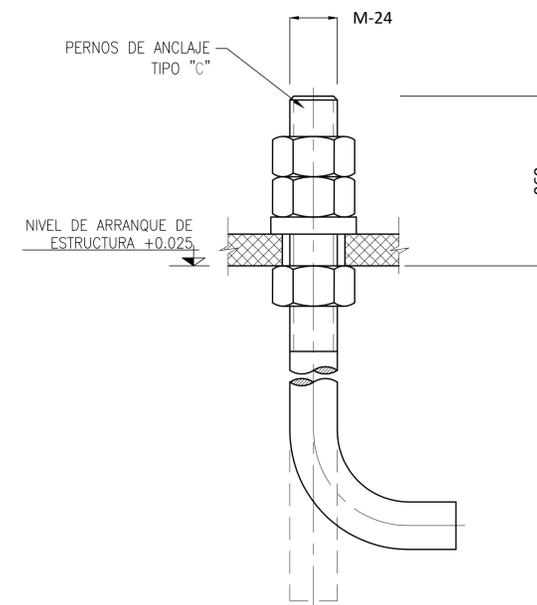
DETALLE PERNO DE ANCLAJE TIPO
