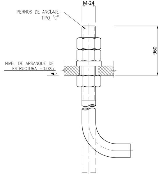
DETALLE PERNO DE ANCLAJE TIPO
