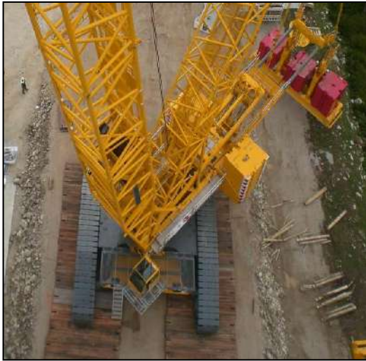
Fig. 27 Wooden sleepers under the crane to prevent excessive ground deformations.
